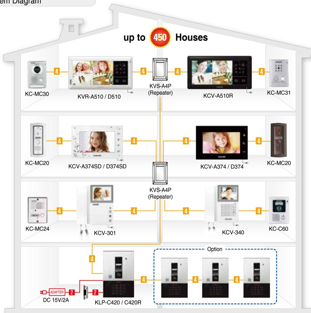
\* Number of extension units for each house is equivalent with the number when the main monitor is used with a door camera for a single house. For example, KCV-A374 supports up to 2 monitors and 2 sub audio phones.
